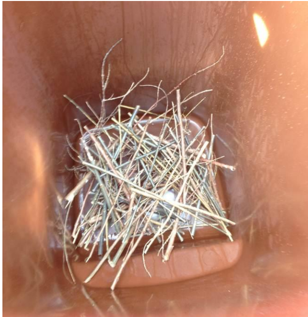
Figure A6.3: Interior of wheelie bin showing the cross hatched twigs at base
