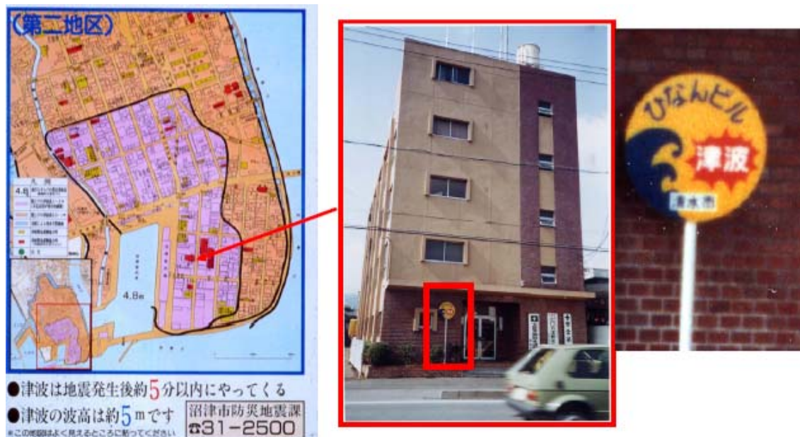
Figure 9 An existing building designated as suitable for vertical evacuation within the high-risk zone and high-density population. The tsunami evacuation signboard is put on the building (Source: Shuto and Fujima, 2009).
