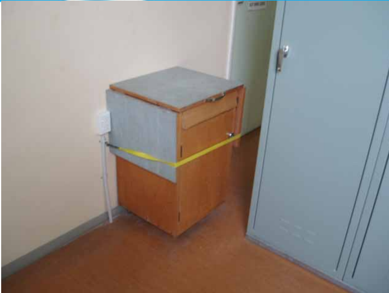
Restrained furniture in relay room (Gisborne prior to earthquake)
